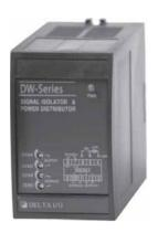
This instrument receives DC voltage and current as an input signal and provides conversion output when the input & output is separated completely. Especially an input, an output and power are isolate using a transformer and it is called "3 ways isolator". this instrument is a high speed response converter like computer interface.
