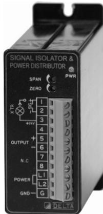
This instrument is a high and accurate converter that has provides all transmitters such as pressure transmitter, flow and overvoltage protection circuit inside with power supply and signal conversion. It is totally isolated between input signal from transmitter and output signal of a converter so it does not need extra isolator when the loop is constructed.
