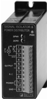
This instrument receives DC voltage and current as an input signal and provides conversion output when the input & output is separated completely. It especially selects 3ways isolation circuit of which input and output are separated by transformer and power and input/output by transformer.
