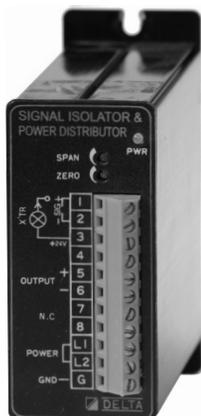
This converter is possible to limit output range to high/low limit 0~100% as being Input of DC voltage and current output signal. It is used in limit control system in combination with output signal of main controller.
