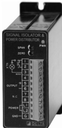
This instrument is a high and accurate converter that receives resistance signals of 3 wires potentiometer (100Ω ~ 100KΩ) and converts them into DC voltage and current. Especially, it is widely used for float type water level detector, and mutual interference by Zero adjustment and Span adjustment is hardly occurred.
