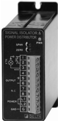
This instrument is a high accurate converter that receives various T/C as an input signal and converts the TC temperature into DC current and DC voltage through the temperature compensation and linear circuit that correspond to the various T/C. Input, output and power have isolation circuit that is separated from each other.
