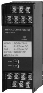
This device is a compact type of high accuracy signal Converter with power supply that supplies DC power to 2wire transmitters and derives 4~20mA of DC signal from the DC power as an input, and then outputs the isolated DC voltage & DC current.
