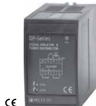
This instrument is a high accurate converter that provides simultaneously all transmitters such as pressure transmitter, flow transmitter, and level transmitter with power supply and signal conversion. Also, it contains overcurrent and overvoltage protection circuit inside. It is totally isolated between input signal from transmitter and output signal of a converter so it does not need extra isolator when the loop is contructed.
