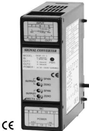
This instrument receives DC voltage and current as an input signal and provides conversion output when the input & output is separated completely. Especially, an input, an output, and power are isolated using a transformer and it is called 3ways isolator.
