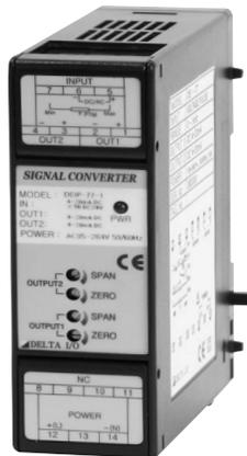
This instrument has alternating sinusoidal voltage as an input, and then calculates as average value and converts it into DC signal proportional to an effective value of input.
