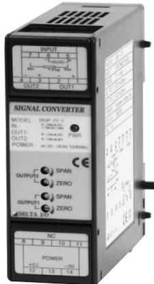
This instrument receives DC voltage and current as an input signal then reverse output signals of all instrument if the reverse is needed. Especially, an in, an output, and power are isolated by a transformer and it is called "3 ways isolator". Power adopts free voltage. In the mounting method is DIN RAIL mounting.
