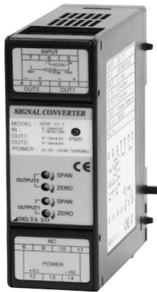
This instrument has alternating sinusoidal current as an input, and then calculates as average value and converts it into DC signal proportional to an effective value of input.
