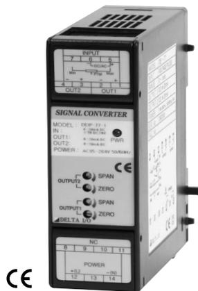
This instrument is a high and accurate converter that receives RTD as an input signal then converts resistance variations into DC voltage and DC current output signal following the temperature. Also the feed back circuit developed by our company actualized high accurate linearization and compensation of line resistance. Power adopts free voltage. In the mounting method is DIN RAIL mounting.
