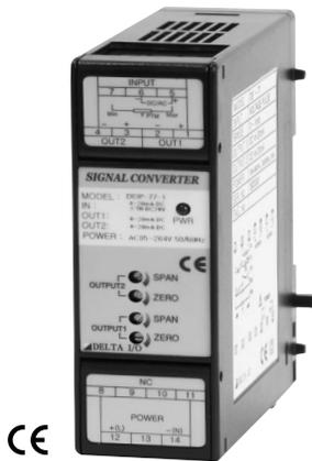
This instrument is a high and accurate converter that receives resistance signals of 3 wires potentiometer (100Ω ~ 100kΩ) and converts them into DC voltage and current. Especially, it is widely used for float type water level detector. And mutual interference by zero adjustment is hardly occurred.
